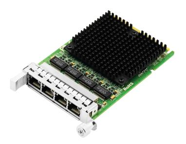
LRES3019PT-OCP is a OCP3.0 SFF Quad-port copper gigabit ethernet network adapter developed by Shenzhen Lianrui Electronics Co., Ltd. based on Net-swift. The adapter card achieves a four-port bidirectional communication transfer rate with a theoretical throughput of 8G on a PCI Express v2.1 x4 bus.
